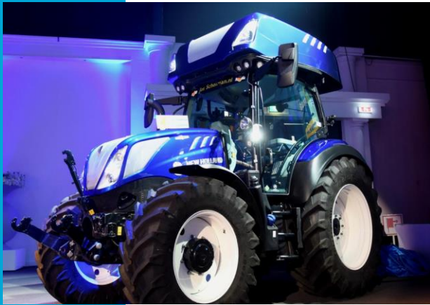
JosScholman/New-Holland: Tractor, dual fuel (diesel+H 2 )
