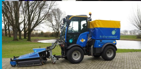
Dual Fuel Tractor and Holder; 60-80% hydrogen in diesel engine
