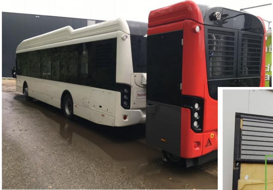
Fig. 10: VDL Citea test vehicle with GiantLeap FC range extender trailer
